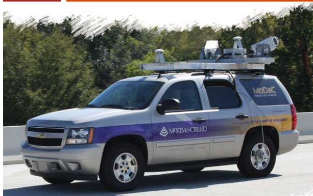
Sporting two lidar sensor heads, the rooftop mobile scanning system collects data while traveling at posted speeds.
